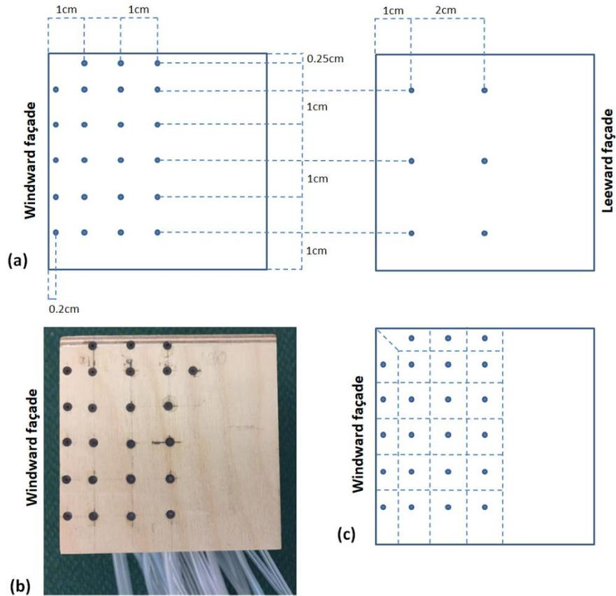
**Fig. 4.** a, b) Pressure taps position at windward and leeward façades of the target cube. c) Sub-areas of the windward façade employed for the calculation of the drag force via the pressure-derived method.
