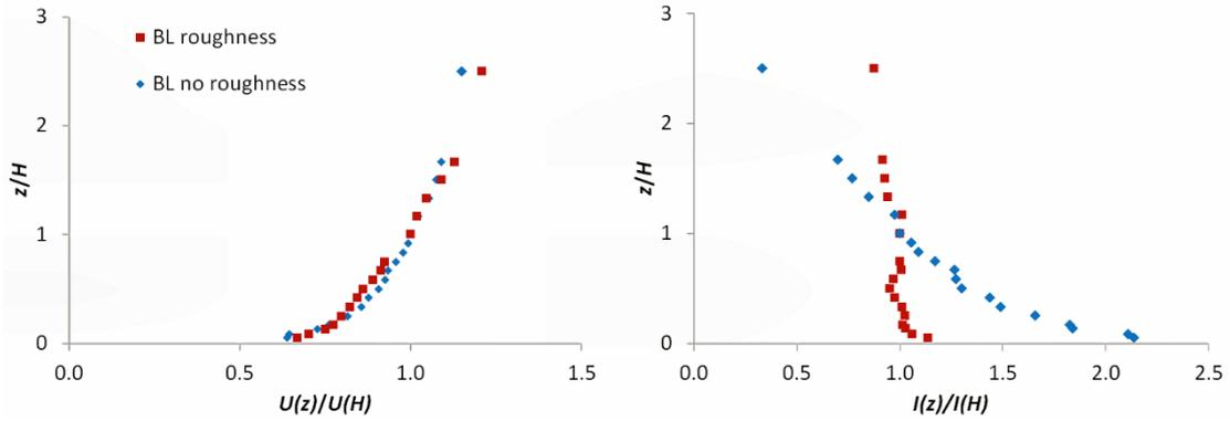
**Fig. 2** a) Boundary layer (BL) wind velocity (left) and relative turbulence intensity (right) incoming profiles in the wind tunnel for rpm = 500. The profiles have been fitted using power laws in Eqs. 1, 2 and 3.
