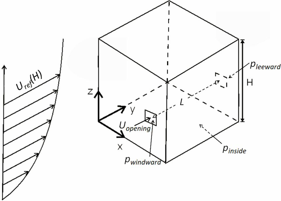
**Fig. 5.** A cube with two openings located opposite to each other.
