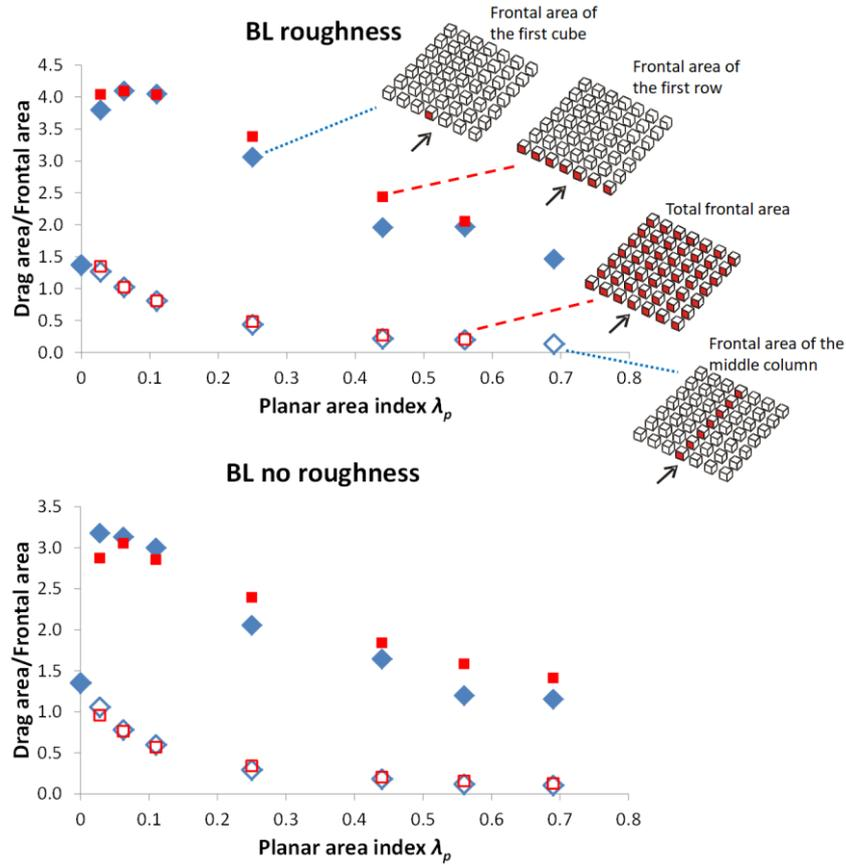
**Fig. 8.** Drag area/Frontal area as a function of the planar area index  $\lambda_p$  when using the frontal area of the first cube or of the first row of cubes (full rhombus and square, respectively) and the frontal area of the middle column or of all the cubes (empty rhombus and square, respectively) in the a) “BL roughness” and b) “BL no roughness” cases. Note: square symbols refer to drag force measurements over the whole array (Buccolieri et al., 2017).
