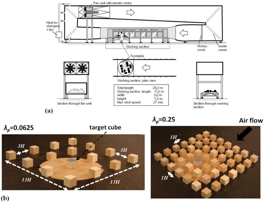
**Fig. 1** a) Sketch of the wind tunnel. b) Example arrays with planar area index  $\lambda_p=0.0625$  and  $0.25$ , with indication of air gap between cubes and the target cubes (roof s highlighted in grey) placed in the centre of the turntable along the centre of the arrays.
