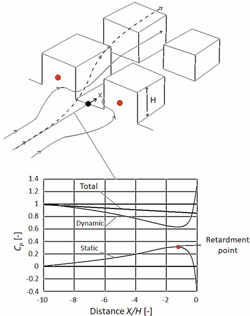
**Fig. 6.** Flow towards the cubes in the front row. a) Sketch of the flow pattern and b) pressure coefficient by static, dynamic and total pressure along the line indicated in a) (adapted from Sandberg et al., 2004).
