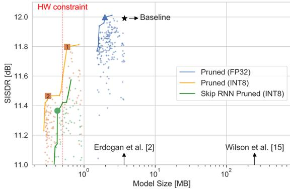
Figure 1: *MS vs. SISDR*. Each point represents a model checkpoint and lines represent a Pareto front.
