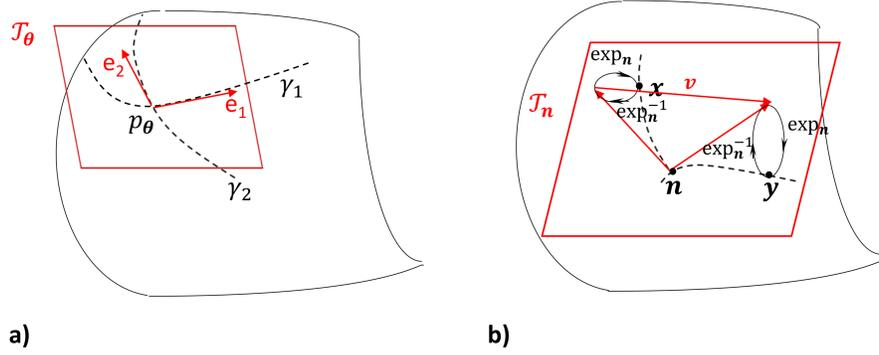
**Fig. 1** a) A manifold (in black) and its tangent space in point  $p_\theta$  (in red) where two coordinate curves (dashed lines) are crossing. The velocities of the coordinate curves are the basis vectors  $e_1$  and  $e_2$ . b) Exponential map and its inverse via the tangent space anchored in a reference point  $n$ . The points  $x$  and  $y$  are mapped via  $\exp_n^{-1}$  to the tangent space. The difference vector between the two mapped points is  $v = \text{vec}(x, y)$ .
