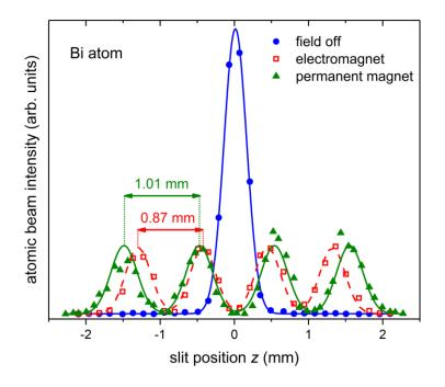
**Figure 4.** Magnetic deflection experiments on an atomic Bi beam using electromagnet (dashed red line) and permanent magnet (solid green line) deflectors. The beamlet data points for each measurement are fitted with four identical equidistant Gaussian functions. With the apparatus dimensions given in the text and Eq. (1), field gradients of 305 T/m and 334 T/m are deduced for the electro- and permanent-magnet units, respectively.
