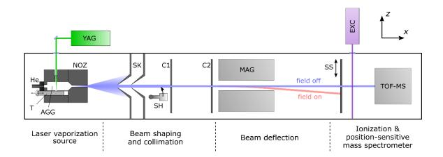
**Figure 3.** Outline of the magnet calibration experiment. NOZ: nozzle, He: helium pulsed valve, YAG: frequency-doubled Nd:YAG laser, T: target rod, AGG: aggregation chamber, SK: double skimmer, SH: shutter, C1 and C2: collimators, MAG: deflection magnet, SS: scanning slit aperture, EXC:  $F_2$  excimer laser, TOF-MS: time-of-flight mass spectrometer.
