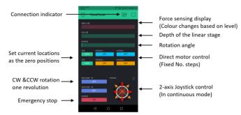
Fig. 4. Screenshot of the robot control software developed in Blynk.
