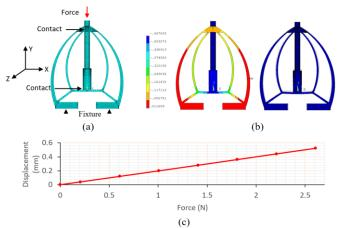
Fig. 5. FE modeling of the swab gripper when subjected to external forces: (a) the mesh results with the force, contacts, and the boundary conditions shown, (b) the displacement results under 2.50N, and (c) the force-displacement relationship with the forces applied from 0 to 2.50N.
