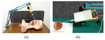
Fig. 7. Experimental setups for (a) the phantom and (b) the pig nose tests.
