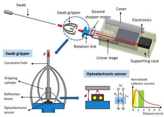
Fig. 2. Schematic illustration of the proposed 2-DOF active end-effector with each component and the mechanism of the force sensing swab gripper shown.
