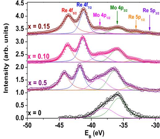
FIG. 1. X-ray photoelectron spectroscopy of the  $\text{Mo}_{1-x}\text{Re}_x$  alloys corresponding to the  $\text{Re}5p$ ,  $\text{Mo}4p$  and  $\text{Re}4f$  inner core shells having binding energies within the range -30 to -50 eV. The symbols represent the experimental spectra and the lines are the multi-peak fits used to extract the peak positions.
