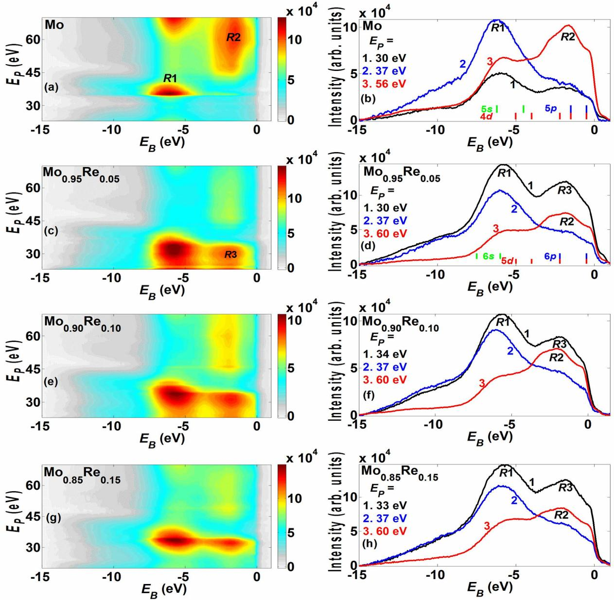
FIG. 2. Photoelectron spectra of the valance band of  $\text{Mo}_{1-x}\text{Re}_x$  at room temperature for (a,b)  $x = 0$ , (c,d)  $x = 0.05$ , (e,f)  $x = 0.10$  and (g,h)  $x = 0.15$ . The images in the left are contour plots while the graphs in the right are photoemission spectra at a few selected  $E_P$ . Two resonances are seen in Mo while three resonances are observed in the alloys.
