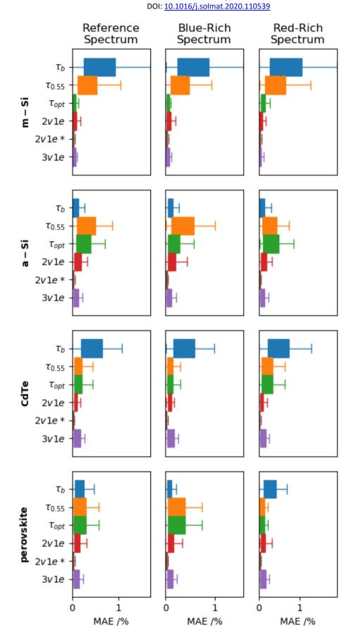
Fig. 13. Boxplots representing the mean absolute errors (MAE) found after 1000 iterations in which the soiling ratios,  $r_s$ , are modelled by introducing a random error of  $\pm 0.5\%$ , at each wavelength, for the transmittance spectra used as input, compared to the soiling ratios calculated from the original spectra. The 2v1e and the 3v1e
