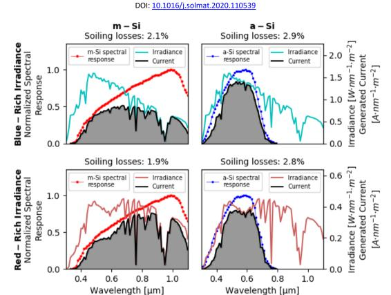
Fig. 2. Soiling losses recorded for Measurement A (shown in Fig. 1, with an average transmittance loss 2.7%) for m-Si and a-Si cells under red-rich or blue-rich irradiance conditions. Each plot shows the spectral response (left axis), the irradiance and the generated current (right axis) for a different combination of irradiance and PV material. The shaded area is the integral in the numerator of Eq. (2).
