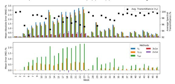
Fig. 6. MAE and ME comparing the measured spectral transmittance with the flat transmittance profiles modelled using the average transmittance ( $\tau_{avg}$ ), with the transmittance at 0.55  $\mu$ m ( $\tau_{0.55}$ ) and the transmittance at the optimal wavelength ( $\tau_{opt}$ ) approaches, and with the spectral transmittances modelled using the three-variable single exponential (3v1e), and the two-variable single exponential (2v1e) methods.
