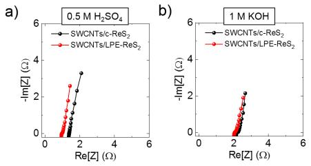
**Figure S11.** Nyquist plots SWCNTs/c-ReS<sub>2</sub> and SWCNTs/LPE-ReS<sub>2</sub> obtained by EIS measurements at open - circuit potential from 0.1 Hz to 200 kHz in (a) 0.5 M H<sub>2</sub>SO<sub>4</sub> and (b) 1 M KOH.
