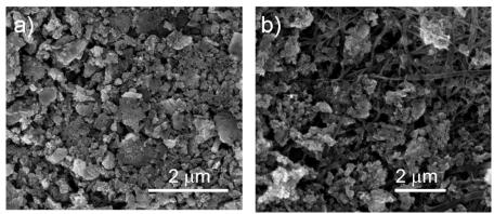
**Figure S9.** Top-view (a) and cross sectional (b) SEM images of SWCNTs/ c-ReS<sub>2</sub>, revealing a partial penetration of ReS<sub>2</sub> crystals into the SWCNT network.
