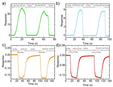
**Figure S7.** Representative stability-retention tests on devices fabricated with MPA-exchanged c-ReS<sub>2</sub> under 10s steps for different target gases, (a) NH<sub>3</sub>; (b) H<sub>2</sub>O; (c) ethanol and (d) acetone, combining 3 steps: (i) gas inlet; (ii) gas flow paused (noted as 'env.') and (iii) N<sub>2</sub> cleaning. The gas-induced response was determined from the film conductance variation as detailed in the main text  $[(G_{gas} - G_{inert})/G_{inert}]$ .
