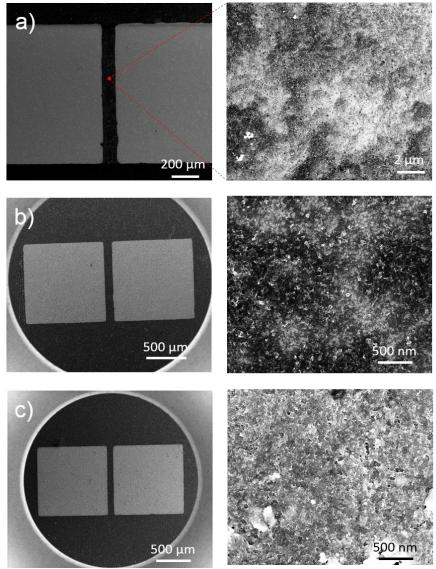
**Figure S6.** (a) Representative SEM images of a device fabricated with MPA-exchanged c-ReS<sub>2</sub>, in which the film was prepared by spin coating method highlighting the formation of holes in the film. (b, c) Representative SEM images of gas sensors built with ABA- and BDT-exchanged c-ReS<sub>2</sub>, in which the film was prepared by drop-casting method showing a homogeneous film (thickness of about 400 nm), respectively.
