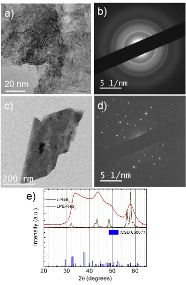
**Figure S3.** (a, c) BF-TEM images and (b, c) corresponding SAED patterns of (a, b) an aggregate of c-ReS<sub>2</sub> nanosheets and (c, d) a flake in the LPE-ReS<sub>2</sub> sample. (e) The background-subtracted and azimuthally integrated SAED patterns, plotted as a function of the Bragg angle calculated for Cu K $\alpha$  wavelength, are compared to the powder XRD pattern for triclinic ReS<sub>2</sub> (ICSD structure n. 650077).
