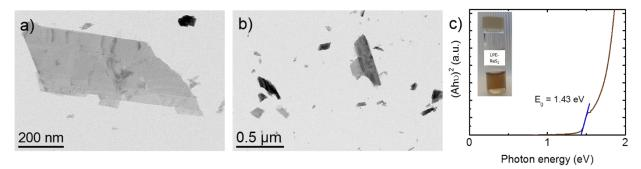
**Figure S2.** (a,b) Representative TEM images of the LPE-ReS<sub>2</sub> flakes. (c) Tauc plot of the LPE-ReS<sub>2</sub> sample with the corresponding fitting for the estimation of the  $E_g$ . The inset shows a photograph of the LPE-ReS<sub>2</sub> dispersion in IsOH.
