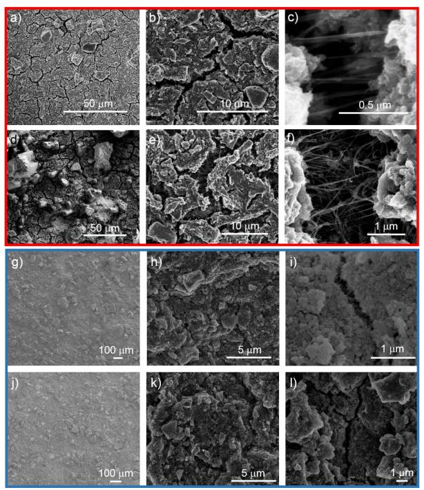
**Figure S13.** Top-view representative SEM images at different magnification of the SWCNTs/c-ReS<sub>2</sub> electrodes after stability test 24 h (red square, a-f) and 48 h (blue square, g-l) for HER in 0.5 M  $H_2SO_4$  (a, b, c, g, h, i) (the enlargement increases from right panels to left panels) and in 1 M KOH (d, e, f, j, k, l) (the enlargement increases from right panels).
