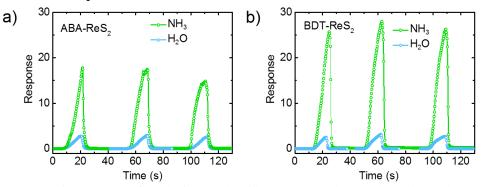
**Figure S8.** Representative response of the devices made with ABA- (a) and BDT- (b) exchanged c-ReS<sub>2</sub> under the presence of NH<sub>3</sub> and moisture (H<sub>2</sub>O). The gas-induced response was determined from the film conductance variation as detailed in the main text  $[(G_{gas} - G_{inert})/G_{inert}]$ .
