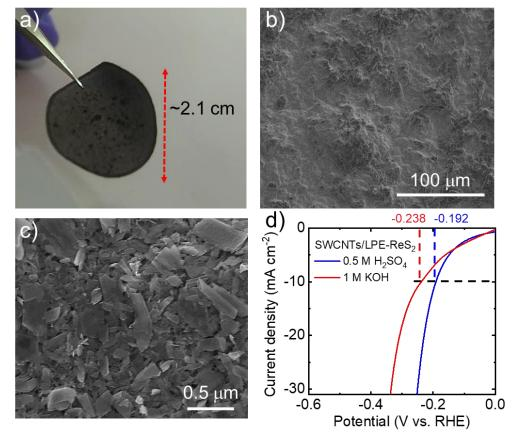
**Figure S10.** (a) Top-view photograph of SWCNTs/LPE-ReS<sub>2</sub> (electrode area: ~3.5 cm<sup>2</sup>). (b-c) Top-view SEM images of SWCNTs/LPE-ReS<sub>2</sub>. (d) iR-corrected polarization curves of the SWCNTs/LPE-ReS<sub>2</sub> in acidic (0.5 M H<sub>2</sub>SO<sub>4</sub>) and alkaline (1 M KOH) media. The  $\eta_{10}$  values are also indicated.
