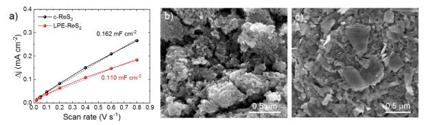
**Figure S12.** a) Scan rate dependence of the  $\Delta j$  calculated form CV curves of c-ReS<sub>2</sub> and LPE-ReS<sub>2</sub> films deposited on GC. The linear fits of the curves and the calculated C<sub>dl</sub> values are also shown. (b, c) Representative SEM images of the as-prepared SWCNTs/c-ReS<sub>2</sub> (b) and SWCNTs/LPE-ReS<sub>2</sub> (c) electrodes showing the arrangement of the c-ReS<sub>2</sub> nanosheets and LPE-ReS<sub>2</sub> flakes, respectively.
