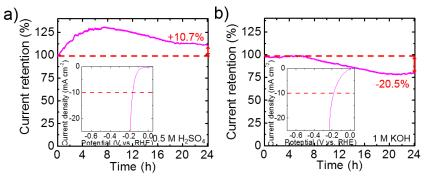
**Figure S14.** (a,b) Chronoamperometry measurements (current retention *vs.* time) for the SWCNTs/c-ReS<sub>2</sub> electrode in acidic (0.5 M H<sub>2</sub>SO<sub>4</sub>) and alkaline (1 M KOH) solutions. A constant overpotential has been applied in order to provid e an equal starting cathodic current density of 20 mA cm<sup>-2</sup>. The inset panels of a) and b) show the iR-corrected polarization curves after stability tests.
