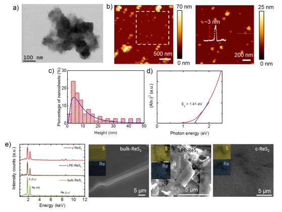
**Figure S1.** (a) Representative TEM image of the c-ReS<sub>2</sub> nanosheets. (b-c) Representative AFM images and heighprofile statistics carried out on 75 assemblies of c-ReS<sub>2</sub> nanosheets (excluding big aggregates). The lognormal fit
