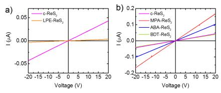
**Figure S5.** (a) I-V characteristics recorded under inert  $N_2$  of the different devices prepared from c-ReS<sub>2</sub> (magenta) and LPE-ReS<sub>2</sub> (orange). (b) I-V characteristics acquired under inert  $N_2$  of the different devices for different ReS<sub>2</sub> nanosheet functionalization: MPA (red); ABA (blue) and BDT (green).
