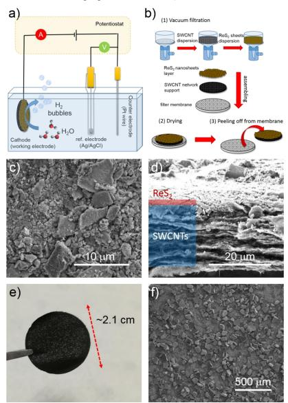
**Figure 5.** (a) Scheme of the electrochemical setup for measuring the electrocatalysts. (b) Sketch of the fabrication of the c-ReS<sub>2</sub>-based electrodes on SWCNTs (c, d) Top-view and cross-sectional SEM images of SWCNTs/c-ReS<sub>2</sub>. (e) Top-view photograph of SWCNTs/c-ReS<sub>2</sub> (electrode area: 3.5 cm<sup>2</sup>). (f) Top-view SEM image of SWCNTs/c-ReS<sub>2</sub> at higher magnification compared to the one shown in panel c (scale bar: 500 μm).
