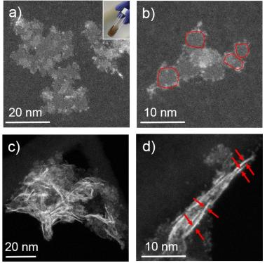
**Figure 1.** Representative HAADF-STEM images of the c-ReS<sub>2</sub> nanosheets, showing (a-b) nanosheets lying mainly parallel to the support film, with individual domains highlighted in (b). In (c,d) the nanosheets lie mainly perpendicular to the carbon support film, as clarified in (d) by arrows pointing at nanosheets viewed along their side. The inset in (a) shows a photograph of the c-ReS<sub>2</sub> dispersion in toluene.
