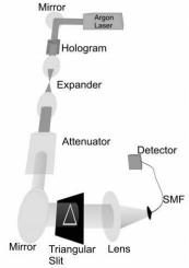
Fig. 4: Sketch of the experimental setup. The light from an Argon Laser acquires an specific OAM state after passing through a computer-generated hologram, before having its intensity strongly attenuated. The photons of this optical field illuminates the triangular slit before being detected, after which a lens and a single mode fiber (SMF) are used for the measurement to materialize in the far-field diffraction limit.
