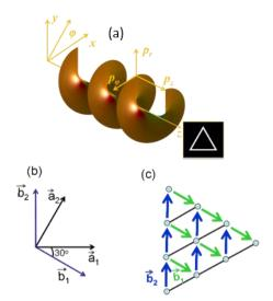
Fig. 1: (a) Schemactical representation of diffraction of a vortex light beam by an equilateral triangular slit. (b) Definition of the direct and reciprocal lattice vectors corresponding to a triangular lattice. (c) Triangular lattice formed with photons with m = 3 of topological charge.
