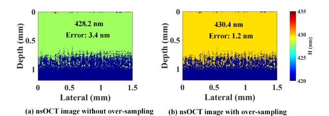
Figure 4. Experimental results of the Bragg grating with axial periodicity of 431.6 nm. (a) The nsOCT without over-sampling presents a 428.2 nm structural size. Error is 3.4 nm. (b)The nsOCT with over-sampling shows a 430.4 nm structural size. Error is 1.2 nm. The color bar presents the spatial periods with unit nanometer.
