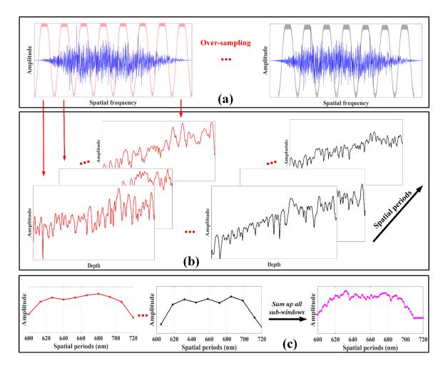
Figure 1. Flowchart for the over-sampling nsOCT signal processing. (a) Decompose axial spatial frequencies into multiple sub-bands and shift the dividing windows for over-sampling the spatial frequencies. (b) FFT of each sub-band and acquire the amplitude along different depths in each particular spatial frequency range. (c) Reconstruct and sum up all the spatial period profiles by taking the energy contribution of each sub-band and then obtain the dominant structural size for each voxel.
