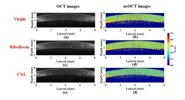
Figure 6. B-scans of *ex vivo* bovine cornea during CXL treatment at three treating steps. (a, b)Both conventional OCT and nsOCT images acquired immediately after epithelial removal. (c, d) Images constructed after 30 min riboflavin instillation and (e, f) after 30 min UVA irradiation while finishing the treatment. The color bar presents the spatial periods with unit nanometer.
