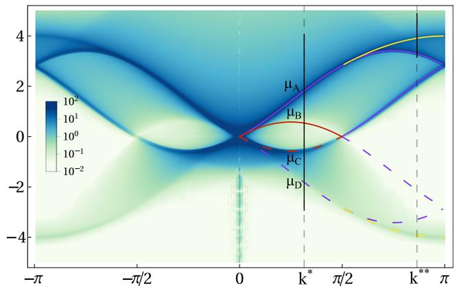
FIG. 2. (Color online) Spectral function of the TG gas on a lattice in the  $(k, \omega)$  plane. Violet, red and yellow lines mark the excitation singularity lines  $\epsilon_1(k)$ ,  $\epsilon_2(k)$  and  $\epsilon_3(k)$ , respectively, which correspond to the elementary processes depicted in the bottom panels of Fig. 1, from left to right, respectively. Parameters used in the calculation:  $N_s = 256$ ,  $N = 64$ .
