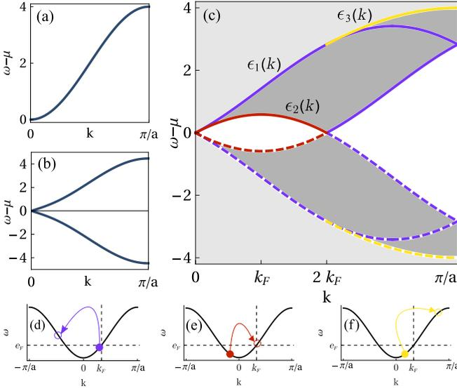
FIG. 1. (Color online) Sketch of the expected spectral function of a Bose fluid on a lattice in the  $(k, \omega)$  plane for (a) zero, (b) weak, and (c) strong interactions. In this work we provide an exact solution for the regime of infinitely strong interaction, which describes generically the case (c). The shaded areas indicate the regions where the spectral function is non-zero. Panels (d), (e) and (f) show the processes that give rise to the singularity lines  $\epsilon_{1,2,3}(k)$ .
