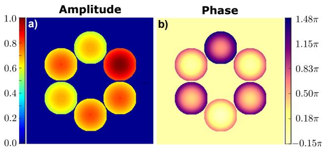
FIG. 3. Initial parameters of the best individual across all runs in the far field test. The amplitude of the beams is shown in a) while the stair step phase profile between any two adjacent beams and curvature of the wavefronts is shown in b).
