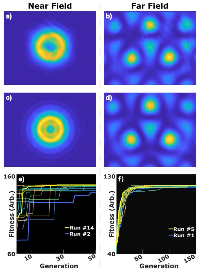
FIG. 2. Results from the GA running on the outer six beams in the far field. The reconstructed intensity profile (b) qualitatively matches the experimental image (a) well with recreating the trefoil-like distribution. The fitness for all generations and runs is shown in c.
