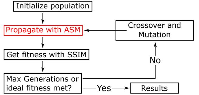
FIG. 1. Block diagram of our GA with the addition of Fourier propagation in red
