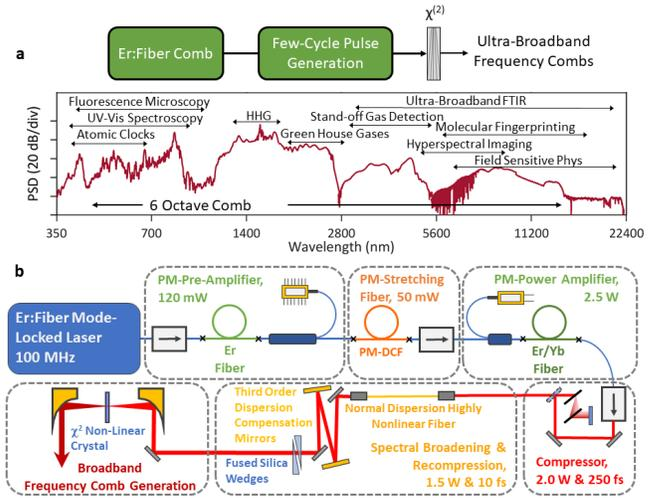
FIG. 1. Generation and applications of a six-octave frequency comb **a**, An erbium (Er) fiber mode-locked laser comb at 1550 nm seeds the generation of a few-cycle pulse to drive frequency conversion in second-order ( $\chi^{(2)}$ ) nonlinear crystals. The resulting composite spectrum spans six octaves for a wide range of applications, as shown. **b**, Schematic of the fiber amplification and short pulse generation. See text for details.
