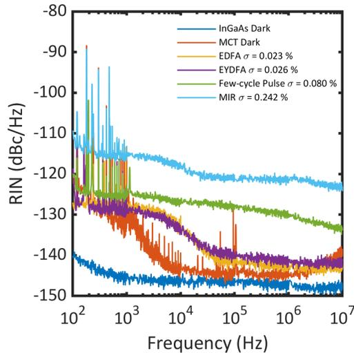
FIG. 5. Measured relative intensity noise of the system.
