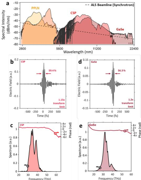
FIG. 4. MIR few-cycle pulses and frequency combs. **a**, Comparison of MIR comb generation from IP-DFG with the Advanced Light Source (ALS) beamline ( $\sim 500$  mA). **b** and **c**, Measured electric field from CSP and the resulting spectrum and phase. **d** and **e**, Measured electric field from GaSe and the resulting spectrum and phase.
