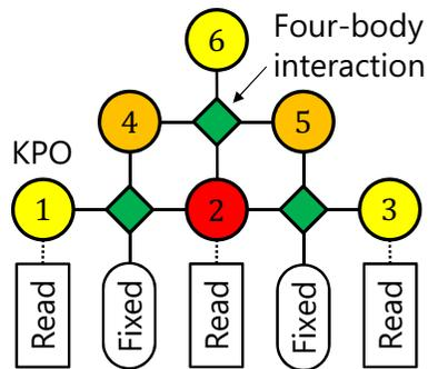
FIG. 1. A network of Kerr-nonlinear parametric oscillators in the Lechner-Hauke-Zoller scheme for the four-spin Ising problem. KPOs 1–6 correspond to LHZ spins  $\tilde{s}_k = \pm 1$ , while the ancillary LHZ spins (“Fixed”) fixed to 1 are implemented by classical driving.
