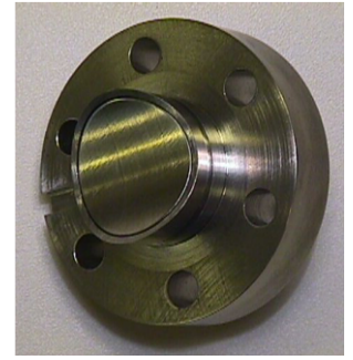
(c) Flange mount LHC button BPM vacuum feedthrough.
