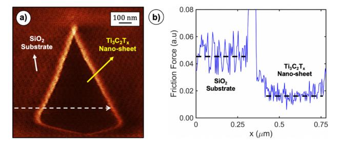
**Figure 2.** (a) Friction map recorded on an isolated, few-layer  $Ti_3C_2T_x$  nano-sheet situated on the SiO<sub>2</sub> substrate. Please note that darker colors correspond to lower friction. (b) Line profile extracted from the friction map of (a) along the dashed white arrow, quantitatively demonstrating the observed friction reduction on the few-layer  $Ti_3C_2T_x$  nano-sheet compared to the SiO<sub>2</sub> substrate.
