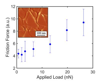
**Figure 3.** Mean friction as a function of the applied load measured on a film comprising multiple  $Ti_3C_2T_x$  nano-sheets. Error bars represent the standard deviation extracted by dividing the corresponding friction map (inset) into a total of ten regions.
