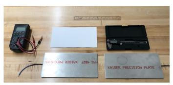
Figure 1: The equipment used to measure  $\epsilon_0$  is shown. Note that the aluminum plates say "PRECISION PLATE", but there was nothing special about these plates. They were pieces of stock that were cut to the same dimensions.
