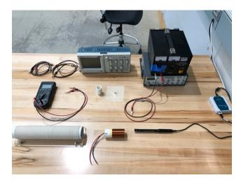
Figure 3: The equipment used to measure  $\mu_0$  is shown. Note that that a signal generator and oscilloscope were provided, but they were not used in the measurements described here.
