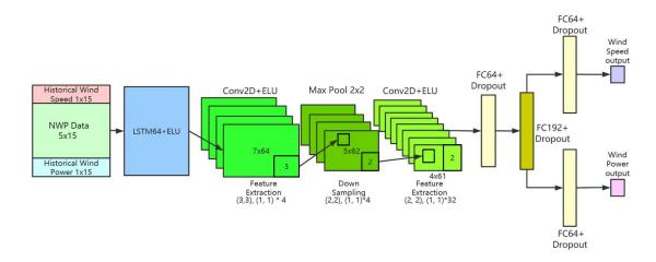
Fig. 2. SIMO model architecture using deep neural networks.
