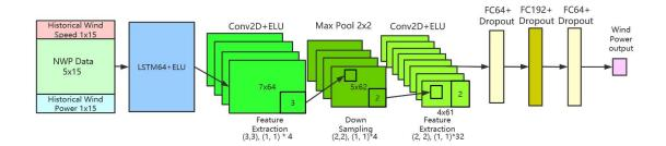
Fig. 1. SISO model architecture using deep neural networks.
