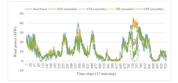
Fig. 10. Ten-day forecasting results in winter case of WF 3 using different ensemble techniques.
