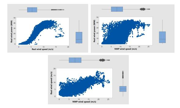
Fig. 3. Marginal plot between real wind power, real wind speed, and NWP wind speed.
