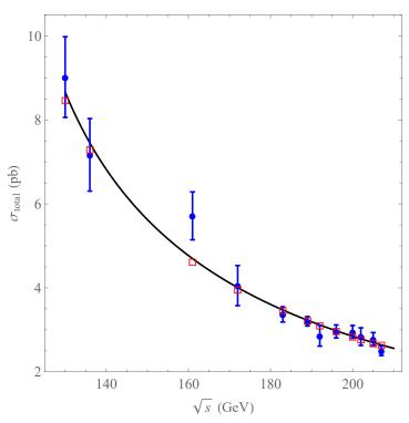
Figure 2: The total cross-section of the process  $e^-e^+ \to \tau^-\tau^+$  as a function of the center-of-mass energy  $\sqrt{s}$ . The LEP-II data and the ZFITTER predictions for the cross-sections are shown as dots with corresponding error bars and red empty squares, respectively [36]. The SM calculation performed using GRACE at the next-to-leading order is represented by the black solid line where  $a_{\tau}^{\rm NP}=0$ .
