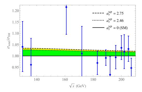
Figure 4: The total cross-section normalized by the SM prediction of the process  $e^-e^+ \to \tau^-\tau^+$  as a function of the center-of-mass energy  $\sqrt{s}$ . The LEP-II data are shown in blue error bars [36]. The SM calculation performed using GRACE at the next-to-leading order is represented by the black solid line where  $a_{\tau}^{\rm NP}=0$ . The dashed and dotted lines correspond to the values  $a_{\tau}^{\rm NP}=2.75$  and 2.46, respectively.
