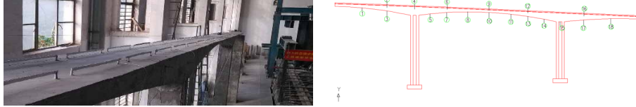
Figure 6: Sensor placement on the scale model of TCRF Bridge.
