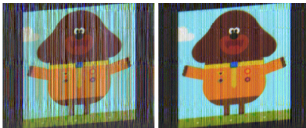
Figure 7: (Left) Reconstructed image using the 256 \times 256 pixels scrambled Hadamard pattern with 1D uniformity correction. (Right) Same reconstructed image using 2D uniformity and contrast correction.
