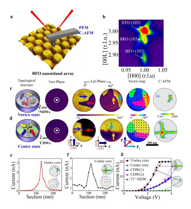
**Fig. 1** Structures of BFO nanoslainds, as well as the domain structures and correspondent conduction patterns for both quadrant vortex and quadrant center topological states confined in two nanoislands. **a,b,** The AFM topographical 3D image of an array of BFO nanoisland (a), and the RSM map for the nanoislands. **c,d,** The domain states and their corresponding C-AFM maps for two topological states: vortex
