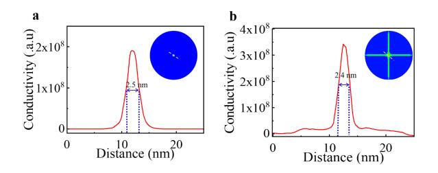
**Supplementary Figure 8** | **The lateral dimension of the conductive topological cores. a,b,** The lateral dimension of the topological cores can be estimated from the full-width at half maxima of the conduction line profiles along the lines for the two topological cores, extracted
