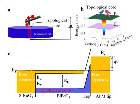
Supplementary Figure 6 | Schematic diagrams of the band structure in the topological core region. a,b, The band bending at the core, creating a conductive channel below the Fermi level. c, The band structure of the conductive core with electrode, under an electric field, wherein an insulating gap exists between the conductive channel and electrode.
