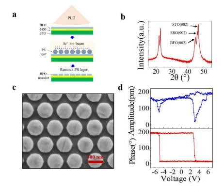
Supplementary Figure 1 | The structural and piezoelectric characterizations of a BFO nanoisland array. a, A schematic flowchart for the fabrication process. b-c, The XRD  $\theta$ -2 $\theta$  scan (b), and the SEM image (c) of the nanoisland array. d, The local piezoresponse butterfly-like amplitude-voltage hysteresis loop and phase-voltage loop on a randomly selected nanoisland.
