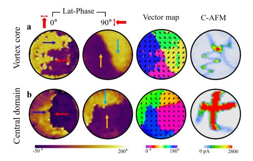
**Supplementary Figure 4** | **The PFM images and domain wall conduction for the two types of topological cores,** *i.e.* vortex state (a) and center state (b), which were selected for further temperature-dependent measurements (see Fig. 2 in the main text). The thin arrows inside the images present the in-plane directions of local polarization component perpendicular to the cantilever. The diameter of each nanoisland is 400 nm.
