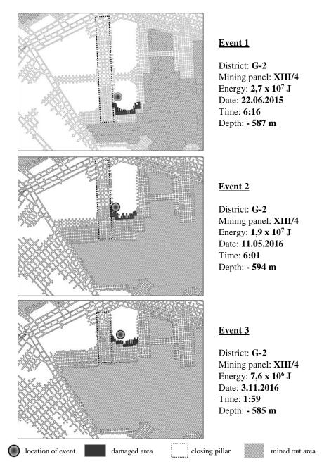
Figure 4. Location of the considered seismic events with the geometry of mining drifts
