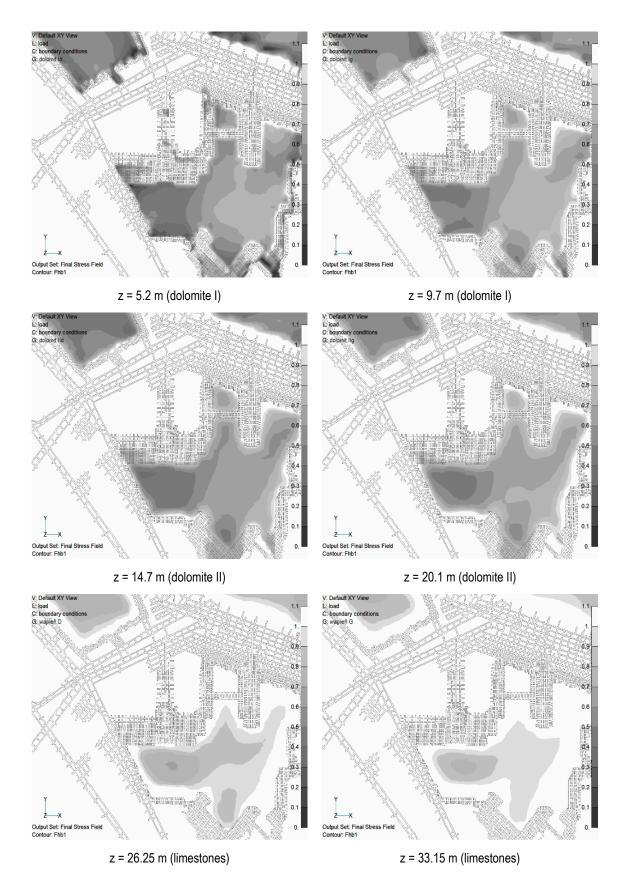
Figure 6. Contours of calculated values of safety factor in the roof strata (event 2)
