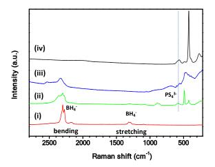
Figure 5. Raman spectra region 2800-210 cm $^{\text{-}1}$  of (i) 3LiBH<sub>4</sub>-LiCl, (ii) LCPS10, (iii) LCPS20 and (iv)  $P_2S_5$  samples.
