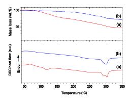
Figure 3. TGA (top) and DSC (bottom) analysis for (a) ball-milled LCPS10 and (b) annealed LCPS10 at 150 °C.
