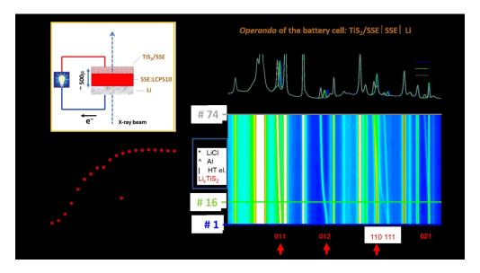
(a) Sketch of the experimental set-up during the operando data record. (b) 2D operando SR-PXD patterns of LCPS10-based battery cell during discharge (partial lithiation of TiS2 electrode, C/10, 60 °C). Selected extracted 1D patterns at different cycling stages are shown on the top. (c) Evolution of the c-axis during lithiation of TiS2. Al foil is used as current collector.
