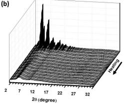
Figure 4. 2D (a) and 3D (b) views of the SR-PXD of the LCPS10 as function of temperature from RT to 150 °C (10 °C min ¹;  $\lambda$  =0.3123 Å). The linear heating scale is shown on the right Y-axis in (a).
