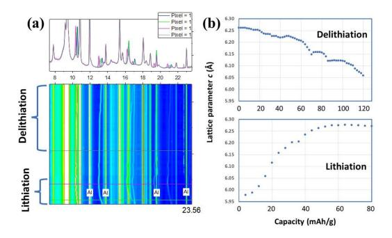
**Figure S2.** (a) 2D *in-operando* SR-PXD patterns of LCPS10-based battery cell during 1 cycle using TiS<sub>2</sub> electrode (extracted 1D pattern is shown on the top); (b) evolution of the *c*-axis during lithiation/delithiation of TiS<sub>2</sub>. The cell was relaxed after lithiation for few hours while the PXD data are continuously collected.
