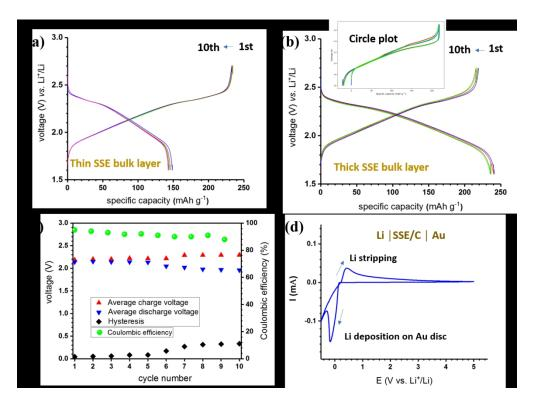
Electrochemical characterization and performance of the LCPS10 SSE: Galvanostatic discharge/charge cycling (0.05 C-rate) at 50 °C with TiS2 electrode (a) using thin (300  $\mu$ m) and (b) thicker (600  $\mu$ m) bulk layer of SSE; For the later cell, (c) average voltage, hysteresis ( $\Delta$ V) and Coulombic efficiency as function of cycle number; (d) cyclic voltammetry at Au disc as working electrode vs. Li+/Li.
