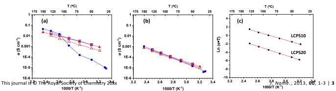
Figure 2. Temperature dependence of the ionic conductivities for (a) LCPS10 and (b) LCPS20 during the first two heating/cooling cycling T ramps. Filled/open squares and triangles correspond to heating/cooling for the 1<sup>st</sup> (blue) and 2<sup>nd</sup> (red) runs, respectively. (c) Arrhenius plots of the 2nd cooling used to infer the activation energies (E<sub>a</sub>) for LCPS10 and LCPS20 samples.
