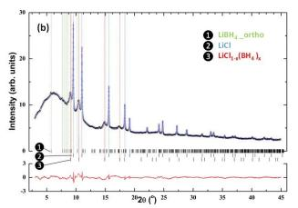
Figure 1. SR-PXD patterns of (a) 3LiBH<sub>4</sub>-LiCl as mixed after ball-milling and (b) LCPS10 solid electrolyte. The collected data at RT are shown in black, the fitted curve in blue, peak markers are shown in order for LiBH<sub>4</sub>, LiCl and LiBH<sub>4</sub>/LiCl, respectively. The difference plot (obs-calc) is shown in red at the bottom ( $\lambda$  = 0.4943 Å).
