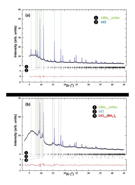
SR-PXD patterns of (a) 3LiBH4-LiCl as mixed after ball-milling and (b) LCPS10 solid electrolyte. The collected data at RT are shown in black, the fitted curve in blue, peak markers are shown in order for LiBH4, LiCl and LiBH4/LiCl, respectively. The difference plot (obs-calc) is shown in red at the bottom ( $\lambda$  = 0.4943 Å).
