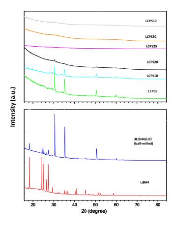
**Figure S1.** Lab-PXD patterns (Cu  $K_{\alpha}$ , 1.5418 Å) of LiBH<sub>4</sub>, ball-milled 3LiBH<sub>4</sub>-LiCl, and in the top figure LiBH<sub>4</sub>-LiCl-P<sub>2</sub>S<sub>5</sub> based mixed systems and further ball-milling with Spex milling; e.g. LCPS5 corresponds to 95(3LiBH<sub>4</sub>/LiCl) - 5P<sub>2</sub>S<sub>5</sub>, and similar for the other compositions.
