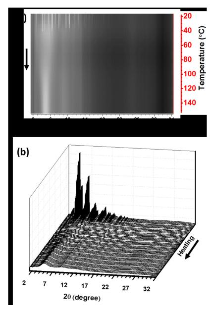
2D (a) and 3D (b) views of the SR-PXD of the LCPS10 as function of temperature from RT to 150 °C (10 °C min-1;  $\lambda$  =0.3123 Å). The linear heating scale is shown on the right Y-axis in (a).
