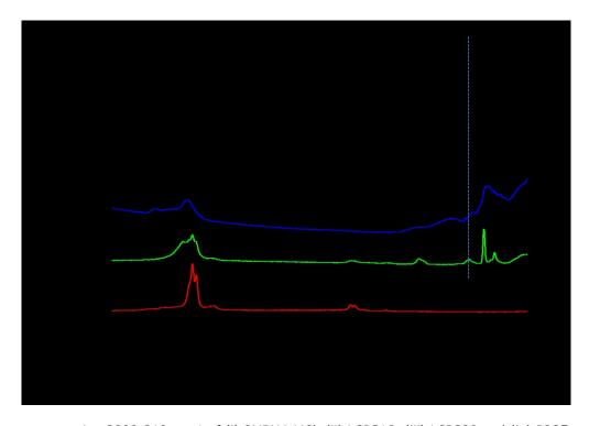
Raman spectra region 2800-210 cm-1 of (i) 3LiBH4-LiCl, (ii) LCPS10, (iii) LCPS20 and (iv) P2S5 samples. 199x139mm~(150~x~150~DPI)
