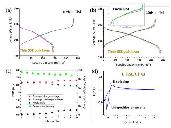
Figure 6. Electrochemical characterization and performance of the LCPS10 SSE: Galvanostatic discharge/charge cycling (0.05 C-rate) at 50 °C with TiS<sub>2</sub> electrode (a) using thin (300  $\mu$ m) and (b) thicker (600  $\mu$ m) bulk layer of SSE; For the later cell, (c) average voltage, hysteresis ( $\Delta$ V) and Coulombic efficiency as function of cycle number; (d) cyclic voltammetry at Au disc as working electrode vs. Li<sup>+</sup>/Li.
