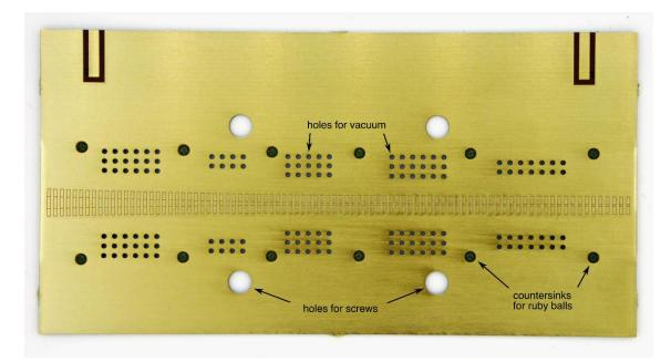
**FIG. S3. Front of the beam splitter's chip.** 270 electrodes arranged in three rows. The width of the inner electrodes changes along the splitter from 0.3 mm to 2.2 mm, while the width of the outer electrodes is 1.4 mm. Countersinks for ruby balls and holes for screws are drilled for alignment and fixation. Additional smaller holes are used to ensure good vacuum.
