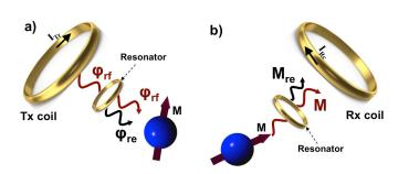
Fig. 1. (a) A passive RF resonator behavior during RF excitation, the resonator locally amplifies transmit field generated by transmit (Tx) coil and resulted in larger transvers magnetization. (b) During the receive phase, magnetization vector (M), which symbolized by a blue spin induces current ( $I_{Rc}$ ) on receive (Rx) coil. Resonator coupling with M and Rx coil results in induced signal amplification.
