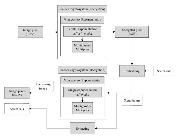
Figure 2. The main components of the proposed steganographic cryptosystem in encryption and decryption processes.
