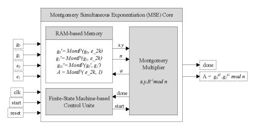
Figure 3. Architecture of the proposed Montgomery Simultaneous Exponentiation (MSE) core.
