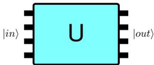
FIG. 1: A photonic device implementing the unitary transformation  $U$  on  $n$  optical modes (black input/output lines):  $|out\rangle = U|in\rangle$ .
