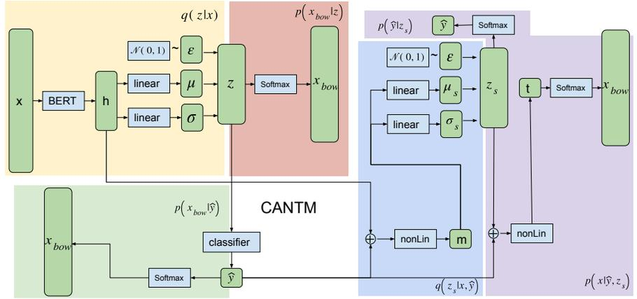
**Fig 1.** Overview of model architecture, linear block is the linear transformation (i.e.  $\text{linear}(x)=Wx+b$ ), nonLin is linear transformation with non-linear activation function  $f(\text{linear}(\cdot))$ , Softmax is Softmax activated linear function
