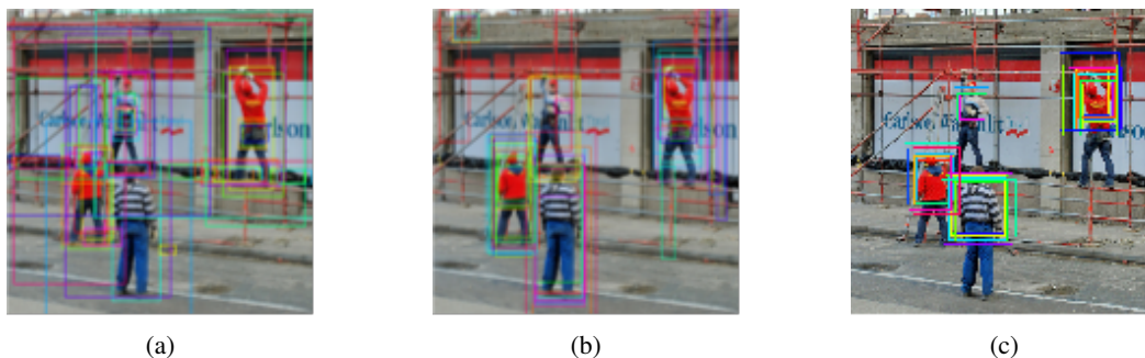
Figure 4: Proposals generated by query “a red shirt” by (a) RPN(COCO) (b) RPN without attention (c) attention-assisted RPN. The bounding boxes are colored only for distinguishing between the dense boxes
