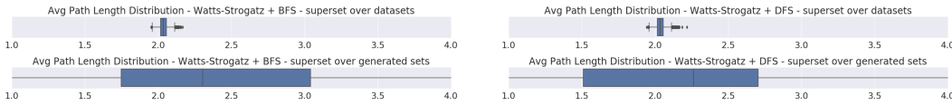
Figure 4: For multiple instances of DeepGG trained on Watts-Strogatz graphs we computed the average path length of each of the 1,000 graphs used for training for both bfs- and dfs-traversal. Equivalently, we computed the average path length of each generated graph from the model (on average 171 for the BFS-instances and 170 for the DFS-instances). Seven DeepGG instances have been trained on bfs-traversals, twelve on dfs-traversals. Watts-Strogatz+BFS constitute a superset in which we generated 1,199 graphs, Watts-Strogatz+DFS a superset in which we computed 2,034 graphs. As to no surprise the average path length distributions for both supersets over datasets are visually equivalent. However, we have to ascertain that the average path length distributions for generated graphs can not only be matched its dataset but also have to point out that the resulting superset distribution for different traversal choices for construction sequences differs significantly.
