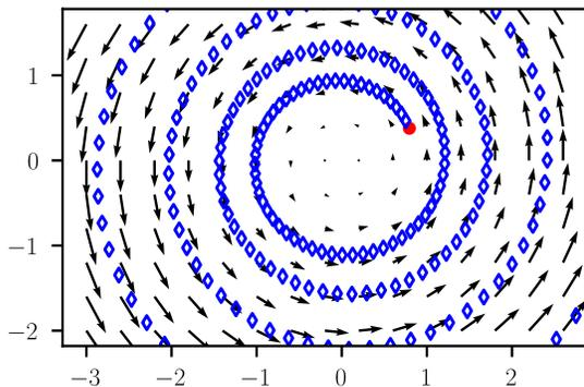
Fig. 1: GDA trajectory for the function  $f(x, y) = xy$ . The iterates of GDA diverge even in this simple scenario. The GDA algorithm starts from the red point and moves away from the origin (which is the optimal solution).
