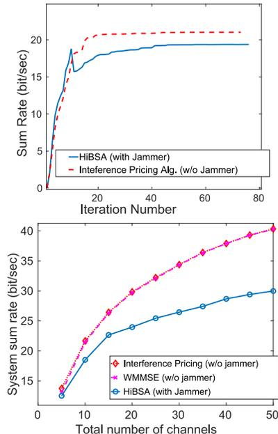
Fig. 2: The convergence curves and total averaged system performance comparing three algorithms: WMMSE, Interference Pricing and HiBSA. All users' power budget is fixed at  $P = 10^{\text{SNR}/10}$ . For test cases without a jammer, we set  $\sigma_k^2 = 1$  for all  $k$ . For test cases with a jammer, we set  $\sigma_k^2 = 1/2$  for all  $k$  and let the jammer have the rest of the noise power, i.e.,  $p_{0,\max} = N/2$ . Figure taken from [19].
