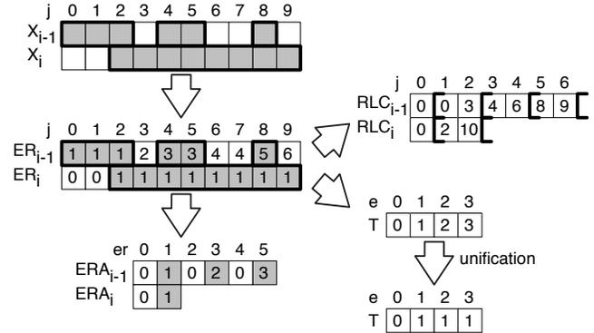
**Fig. 1:** LSL tables for classic foreground labeling: the *even* relative labels corresponding to background components are equivalent to zero in  $ERA$  tables (they will be equivalent to other labels for the proposed foreground and background labeling).
