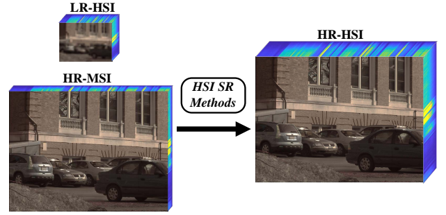
Fig. 1. The illustration of HSI super-resolution from an LR-HSI and an HR-MSI that capture the same scene.
