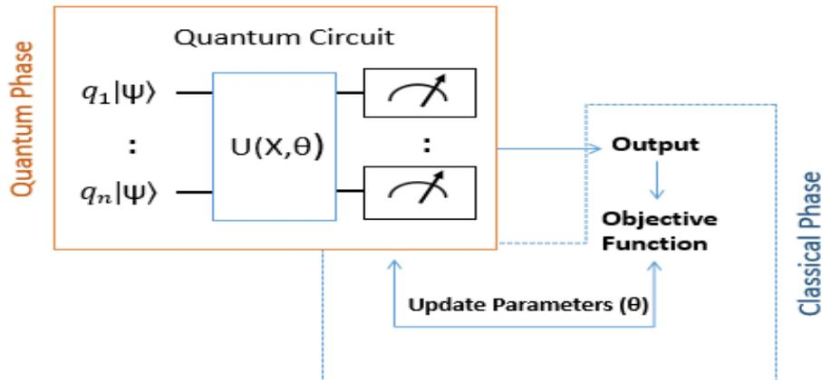
**Figure 1.** Illustration two phases of the variational circuit (parametrized quantum circuit) for Hybrid quantum-classical applications in a quantum machine learning (QML) and quantum neural networks (QNNs). Quantum phase that includes a quantum circuit that consists of state preparation, circuit, and measurement. another phase is a classical phase that includes output after measurement and consists of cost function and learning algorithms which updates parameters ( $\theta$ ).
