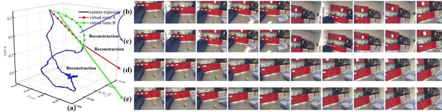
Figure 5: View synthesis based on the Pumpkin dataset by the proposed PoseGANs. (a) camera trajectory of seq-01 in the Pumpkin dataset. (b) corresponding camera shot images along the camera’s trajectory. (c) generated images along the camera’s trajectory. (d) and (e) are images synthesized along virtual routes A and B where the poses along the routes are obtained by linear and parabola interpolations between the start and the end points of the camera’s trajectory, respectively.
