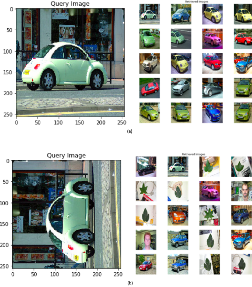
Figure 1: Figure 1: (a) The query image from DB2000[2] is rotationally correct and results precision of 1. (b) The same query image is rotated 90 degrees anti-clockwise and retrieved almost different images resulting precision value of 0.45.
