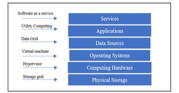
Fig 1: Distribution of Virtualization Layers
