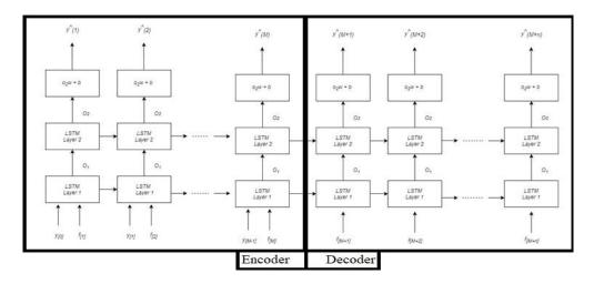
The architecture is divided into two parts: 1) Encoder 2) Decoder shown in Figure 4. The encoder aims to prediction the COVID-19 cases we have already known, yet  $y_{[M-1]}$  and
