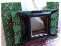
Figure 3: Picture of the MCP-PMT photodetector used for these developments.
