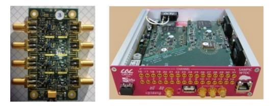
Figure 4: (Left) 4-channels fast amplifier prototype with a 700 MHz bandwidth and a gain of 100 used for the tests described in this work. (Right) 32-channels SAMPIC waveform recorder, which is currently used on many test benches all around the world [SAMPIC Workshop].
