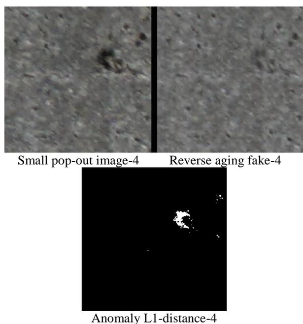
Figure 15. Small pop-out image (upper-left) and reverse aging “health condition fake” (upper-right) translated using trained generator mapping from damaged to normal image. Grayscale L1-distance mask output (bottom).
