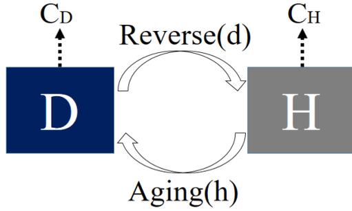
Figure 3. Our applied CycleGAN model mapping functions  $R : D \rightarrow H$  and  $F : H \rightarrow D$ . Discriminator function  $C_D$  classifies whether the image is a real damaged image or a generated fake one, and  $C_H$  discriminates whether it is a real health condition image or a fake output image.
