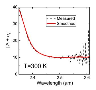
**Figure 4:** Net optical absorption  $(A + \alpha_i)$  spectrum measured by the segmented contact method for a laser emitting at  $\lambda \approx 2 \mu m$ . The observed value of  $\approx 10 \text{ cm}^{-1}$  is higher than the losses typically reported using the inverse cavity length method.
