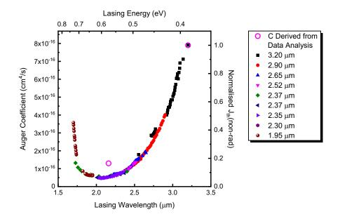
**Figure 5:** Wavelength dependence of the non-radiative threshold current density, with normalisation with respect to two anchor points (open circles) corresponding to Auger coefficients obtained from data analysis with losses derived from optical gain techniques.
