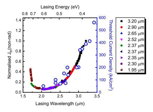
**Figure 3:** Normalised non-radiative threshold current densities (solid points) as a function of lasing wavelength, as obtained from measurements of  $J_{th}$  at high hydrostatic pressure, and using  $J_{rad}$  at ambient as determined from the temperature dependences of  $J_{th}$  and  $J_{rad}$ . The blue open circles are literature values of the total threshold current density taken from Fig. 1.
