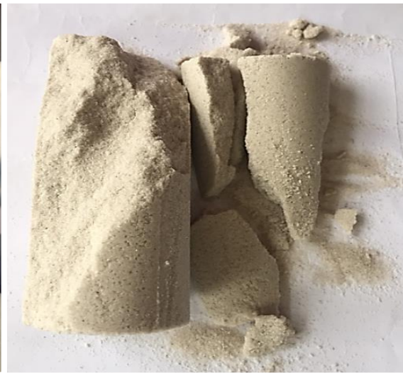
Figure 10 (a) Exemplary photos of samples in the six macro-scale MICP experiments; (b) a photo of an MICP-treated specimen in a UCS test; (c) a photo of the sample after being broken during the UCS test
