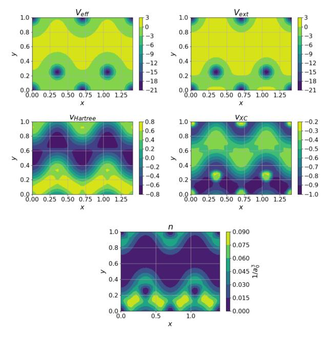
Figure 2: Top: From top left moving clockwise: plot of  $V_{\text{eff}}$ ,  $V_{\text{ext}}$ ,  $V_{\text{XC}}$ , and  $V_{\text{Hartree}}$  in a two-dimensional slice of a Si<sub>2</sub> crystal, along the same plane as the two atoms in the unit cell. Spatial units are in Bohrs ( $5.29 \times 10^{-11}$  m) and potential is in Rydberg units (13.6 eV). Bottom: The resulting electron density (in electrons per cubic Bohr) for the above potential.
