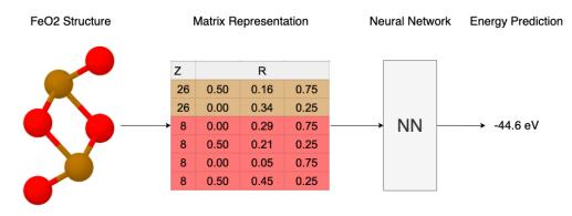
Figure 4: Atomistic neural network approach to predicting material properties. The structure of a material can be represented by a matrix consisting of each atom's atomic number (Z) and its Cartesian coordinates (R) with respect to a reference point. This representation will be used as the input to the neural network, which maps it to a target property, such the exchange-correlation potential of the total energy of the compound.
