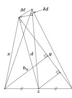
The  $\delta \ell$ -length arc is also the first order hypotenuse of another small right triangle with one leg of length  $\delta d$ , which is similar to the triangle with a d-length hypotenuse and whose corresponding leg is a segment starting from the foot of the median and parallel to – and thus half of the length of – the  $h_y$ -length height, so that
