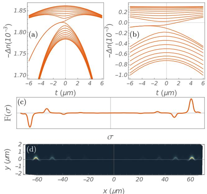
FIG. 4. (Colour on-line) Panels (a,b): The band spectra of  $\Delta n$  vs  $t$  for a chain of 44 combined peaks and troughs terminating with hard walls. Panel (a): Ag-SiO<sub>2</sub>, panel (b): Au-air. Although not clear, there are 20 bands in the plots. Panel (c): the 10th state for either system at  $t = -3 \mu\text{m}$ . Panel (d): the real-space magnetic field amplitude of this very mode.
