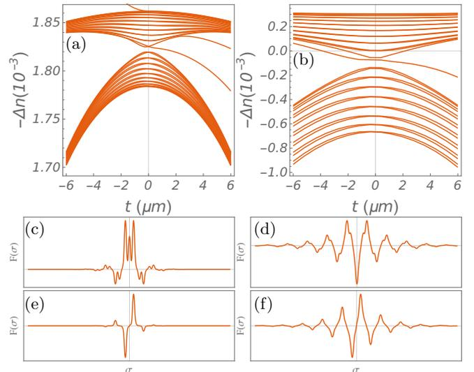
FIG. 5. (Colour on-line) Panels (a,b): The band spectra of  $\Delta n$  vs  $t$  for a chain of 82 combined peaks and troughs within the extended defect-including unit-cell. Panel (a): Ag-SiO<sub>2</sub>, panel (b): Au-air. Panels (c,e): the 21st and 22nd states, respectively, of the Ag-SiO<sub>2</sub> system at  $t = 3 \mu\text{m}$ . Panels (d,f): the 21st state of the Au-air system for  $t = -3 \mu\text{m}$  and  $t = 3 \mu\text{m}$ , respectively.
