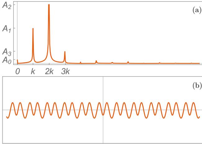
FIG. 2. (Colour online) Panel (a): The Fourier transform of a typical grating profile shows three dominant harmonic modes in its construction. Panel (b): (Not to scale) A plot of the function  $g(x)$  reveals that the bipartite corrugated structure is born from an underlying triharmonic pattern.
