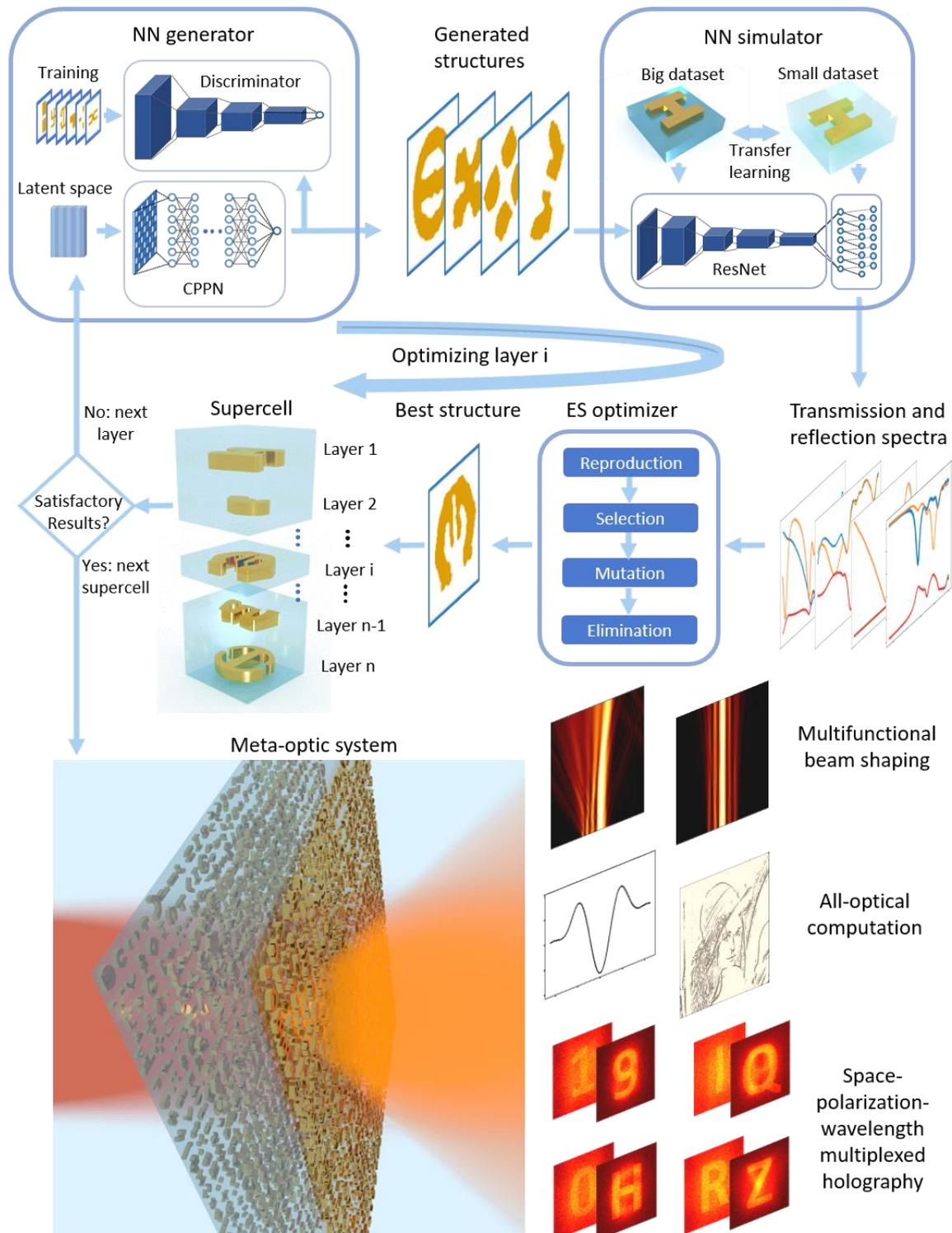
**Figure 1.** Description of the modules of the artificial intelligence (AI) framework. The design flow goes through the neural network (NN) generator, the NN simulator, and the evolutionary strategy (ES) optimizer in a loop. The generator is a Compositional-Pattern Generating Network (CPPN) of a Generative Adversarial Network (GAN). The simulator is trained sequentially through transfer learning. The workflow proceeds as following: the generator first
