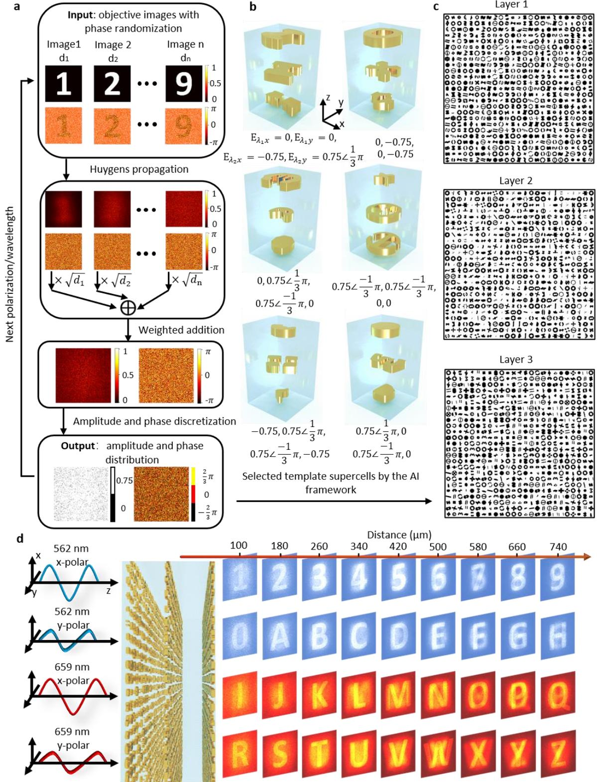
**Figure 4.** AI-designed space-polarization-wavelength multiplexed hologram. The hologram can project 36 different holographic images in total. (a) The flowchart to obtain the amplitude-and-phase distributions of the design objective. The first step is to pin down the target images projected by the hologram and their distances to the hologram plane, then random phases are
