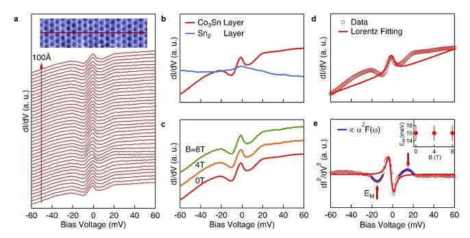
**Fig. 2** Bosonic mode coupling from kagome electrons. a Differential conductance spectra taken along the Co<sub>3</sub>Sn layer shown in the inset. b Spatially averaged dI/dV spectra for Co<sub>3</sub>Sn layer and Sn<sub>2</sub> layer, respectively. c dI/dV spectrum for Co<sub>3</sub>Sn layer taken at different external magnetic fields applied along the *c*-axis. d Fitting of the spectral peak in the Co<sub>3</sub>Sn layer with a Lorentzian. e Second differential
