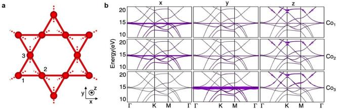
Fig. 5. Vibration nature of the phonon flat band. a, Kagome lattice with dotted lines denoting the directions in which the atomic movement is confined. The inner atoms are displaced according to the elementary localized deformation that comprises the flat band. b, Atom displacement resolved phonon band structure along x, y and z-direction vibration for  $Co_1$ ,  $Co_2$  and  $Co_3$  corresponding to Fig. 5a.
