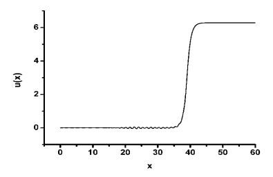
**Fig.2.** The moving kink profile with the oscillating tail in the dispersive sine-Gordon equation at  $\beta = 1/12$  and  $V_{in} = 0.6$ .
