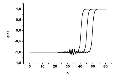
**Fig.4.** The moving kink and the stationary breather mode in the dispersive  $\varphi^4$ -system.
