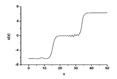
**Fig.5.** The soliton complex dissociation in the case of a small initial velocity ( $V_{in} = 0,3$ ) in the dispersive sine-Gordon equation.
