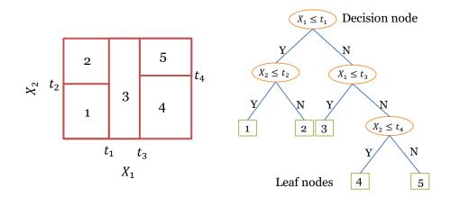
Figure 2.8. Example of a dataset and its corresponding regression tree (Publication III).
