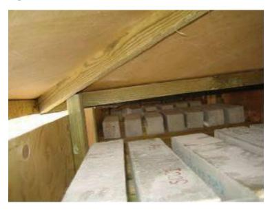
Figure 3.1. Sheltered concrete specimens for carbonation field test (Publication II).
