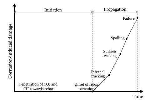
**Figure 2.2.** Corrosion of rebar in concrete structure: initiation and propagation periods (Publication I).
