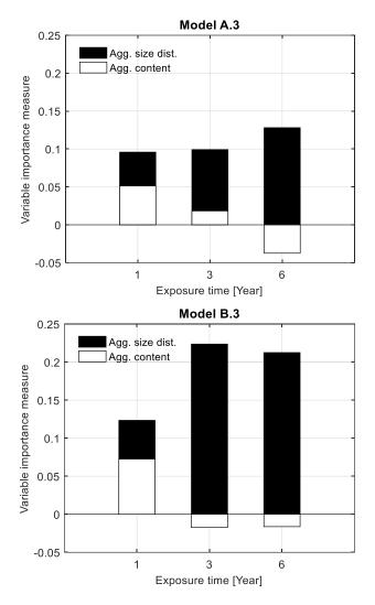
**Figure 4.9.** Significance measure of aggregate size distribution and aggregate content with respect to exposure time in Models A.3 and B.3 (Publication III).
