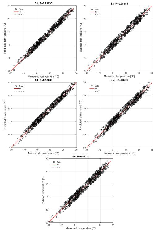
**Figure 4.11.** Training performance of hygrothermal model: inner temperature. Y and T are predicted and measured, respectively.
