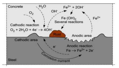
**Figure 2.1.** Schematic illustration of rebar corrosion in concrete as an electrochemical process [19].
