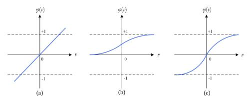
Figure 2.6. Activation functions (a) linear, (b) logistic, and (c) hyperbolic tangent.
